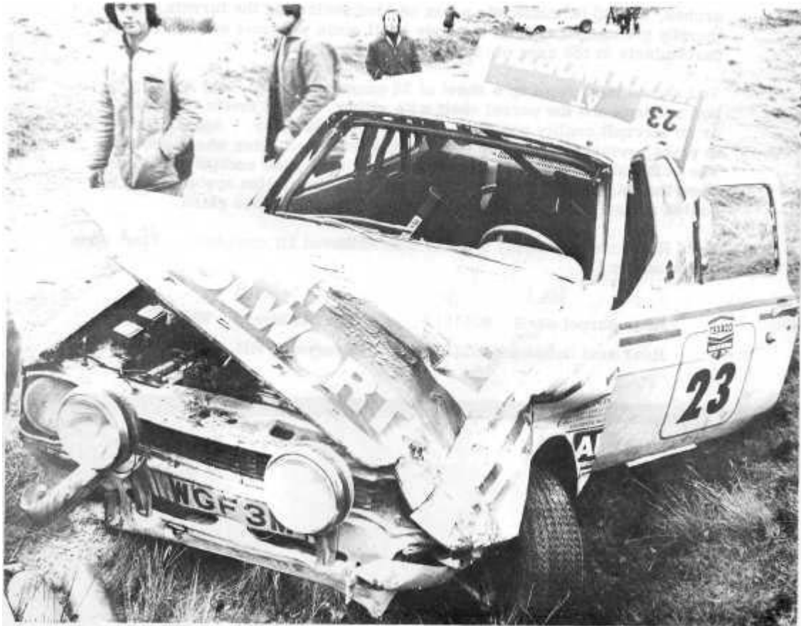
The end of the road for Inurietta's Mk.1 Escort in 1976. Note how roll cage has helped keep the crew compartment in tact.
